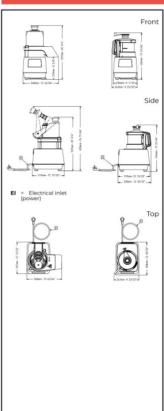
Electric Supply voltage: 220-240 V/1N ph/50 Hz **Electrical power max.:** 0.5 kW 0.5 kW **Total Watts:** Capacity: Performance (up to): 150 kg/hour **Capacity:** 2.6 litres Key Information: External dimensions, Width: 348 mm External dimensions, Depth: 328 mm External dimensions, Height: 527 mm
